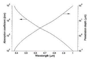
Figure 1 Absorption coefficient and penetration depth in Silicon vs. wavelength.
